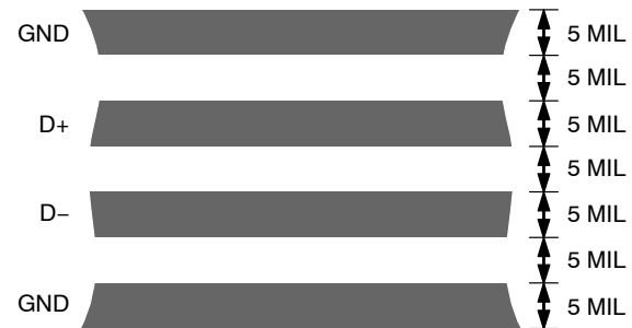
Figure 12. Typical Assignment of Signal Tracks
