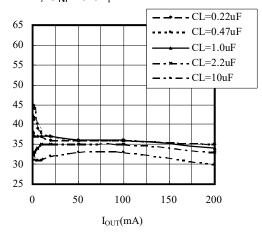
■ Output Noise vs. Output Current C<sub>L</sub> =MLCC, C<sub>NP</sub>=0.01µF
