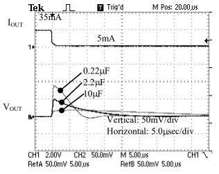
■ Parameter:  $C_L = 0.22 \mu F$ ,  $2.2 \mu F$ ,  $10 \mu F$ Fixed:  $C_{NP} = 0.001 \mu F$
