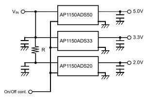
Figure 4. Parallel-Connected On/Off Control
