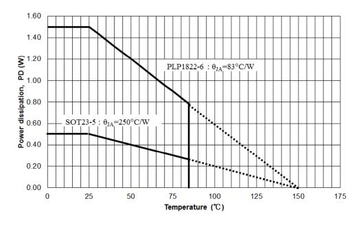
Figure 2. Maximum Power Dissipation
