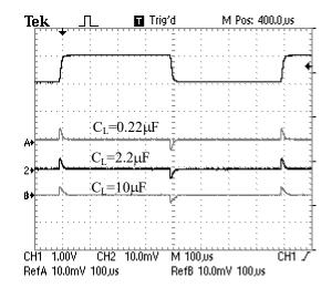
■  $C_{NP}$ =0.001 $\mu$ F, 0.01 $\mu$ F, 0.1 $\mu$ F  $C_L$  =2.2 $\mu$ F
