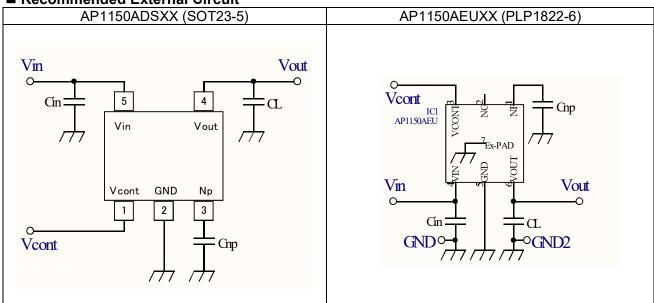
Figure 6. External connection circuit example
