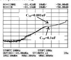
■ Ripple Rejection vs. I<sub>OUT</sub>
