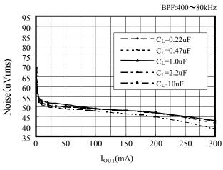
■ Noise vs. Output Current C<sub>L</sub> =MLCC, C<sub>NP</sub>=10000pF
