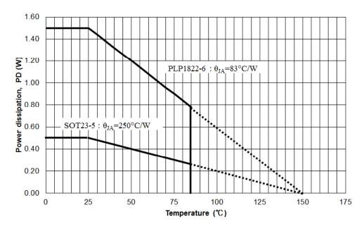
Figure 2. Maximum Power Dissipation
