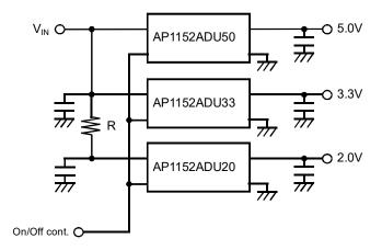
Figure 4. Parallel-Connected On/Off Control
