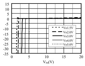
■ V<sub>IN</sub> vs. V<sub>OUT</sub> Regulation Point
