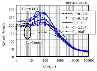
$I_{OUT}$ =30mA,  $C_{NP}$ =10000pF,  $C_{L}$ =0.22 $\mu$ F(MLCC)
