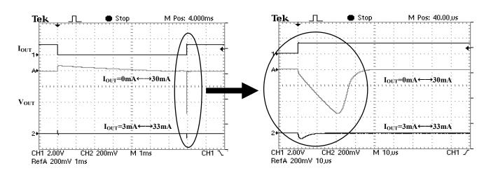
When there is a fast and large current change, please increase the load side capacitor. Please further flowing a little bit of current. Voltage variation can be small.
