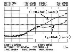
■ Ripple Rejection vs. C<sub>NP</sub>
