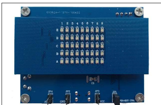
Figure 1: Photo of IS31FL3729 Evaluation Board
