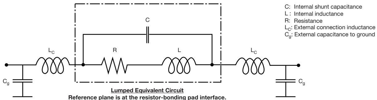
The lumped circuit above was used to model the data at the bonding pad-resistor reference plane. High frequency testing was performed by Modelithics, Inc. on parts mounted to quartz test boards. Quartz test boards were chosen to minimize the contribution of the board effects at high frequencies.
