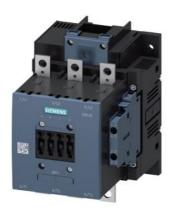
Power contactor, AC-3 185 A, 90 kW / 400 V AC (50-60 Hz) / DC operation 110-127 V UC Auxiliary contacts 2 NO + 2 NC 3-pole, Size S6 Busbar connections Drive: conventional screw terminal
