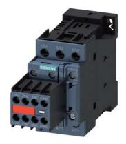
Power contactor, AC-3 32 A, 15 kW / 400 V 2 NO + 2 NC, 24 V DC 3-pole, Size S0 Screw terminal Captive auxiliary switch
