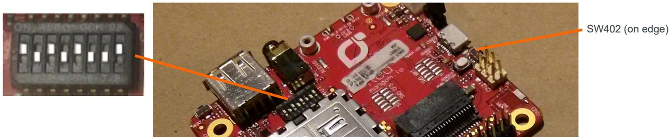
Figure 2-4: SW401 Dipswitch Recommended Settings
