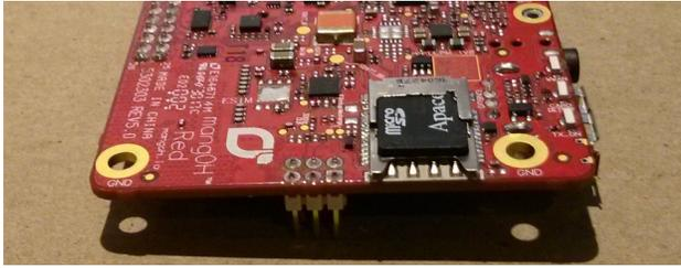
Figure 3-13: microSD—Inserted
