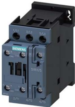
Power contactor, AC-3 32 A, 15 kW / 400 V 1 NO + 1 NC, 220 V AC 50/60 Hz, 3-pole Size S0, screw terminals
