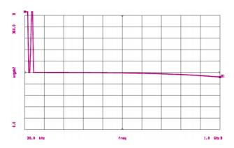
Amplitude Unbalance (5 to -5 dB) vs. Frequency (30 kHz to 1 GHz)
