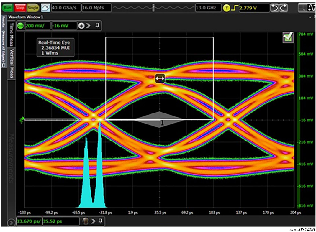
Fig. 11. HDMI 2.1 6 Gbps TMDS eye diagram, PCB with device; typical values
