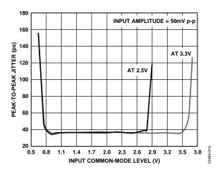
Figure 23. Peak-to-Peak Jitter vs. Input Common-Mode Level
