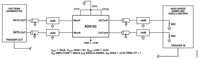
Figure 31. Negative Supply Test Circuit
