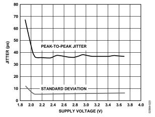
Figure 24. Jitter vs. Supply Voltage
