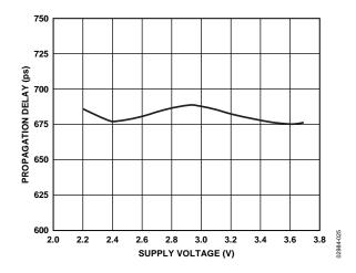
Figure 29. Propagation Delay vs. Supply Voltage
