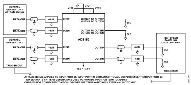
Figure 33. Crosstalk Test Circuit
