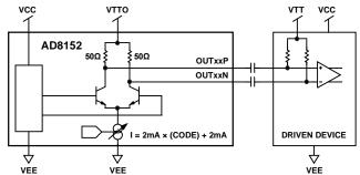
Figure 36. AC Coupling Output Signal from AD8152
