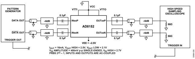
Figure 32. Positive Supply Test Circuit
