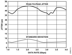
Figure 17. Jitter vs. Data Rate
