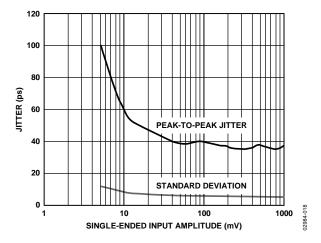
Figure 22. Jitter vs. Single-Ended Input Amplitude
