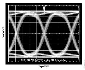
Figure 20. Crosstalk, 3.2 Gbps, Attack Signal On (See Figure 33)
