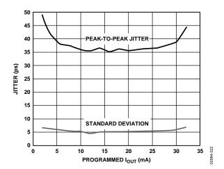
Figure 26. Jitter vs. Programmed IOUT
