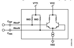
Figure 35. AC Coupling Input Signal from AD8152
