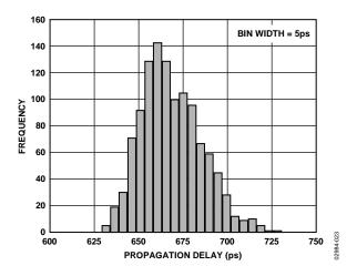
Figure 27. Variation in Propagation Delay
