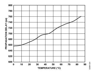
Figure 28. Propagation Delay vs. Temperature
