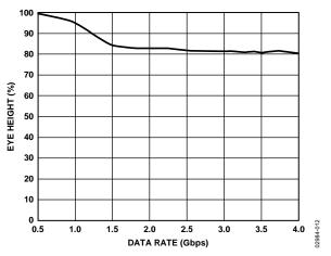
Figure 16. Eye Height vs. Data Rate
