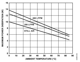
Figure 7. Maximum Power Dissipation vs. Ambient Temperature
