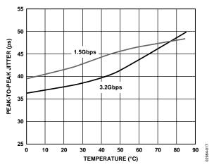
Figure 21. Peak-to-Peak Jitter vs. Temperature
