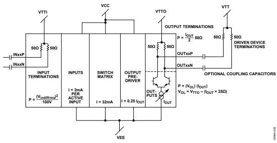
Figure 37. Power Consumption Block Diagram
