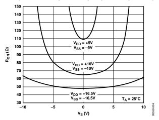
Figure 4. On Resistance ( $R_{ON}$ ) vs. Input Voltage ( $V_S$ ) as a Function of  $V_{DD}/V_{SS}$
