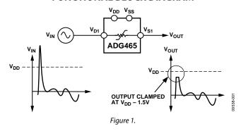
The ADG465 can operate from both bipolar and unipolar supplies. The channels are normally on when power is connected, and open circuit when power is disconnected. With power supplies of  $\pm 15$  V, the on resistance of the ADG465 is 80  $\Omega$  typical, with a leakage current of  $\pm 1$  nA maximum. When power is disconnected, the input leakage current is approximately  $\pm 0.005~\mu A$  typical.
