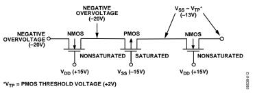
Figure 18. Negative Overvoltage on the Channel Protector
