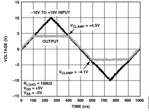
Figure 6. Overvoltage Ramp
