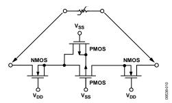
Figure 14. Channel Protector Circuit Schematic
