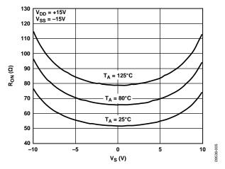
Figure 5. On Resistance ( $R_{ON}$ ) vs. Input Voltage ( $V_{S}$ ) as a Function of Temperature
