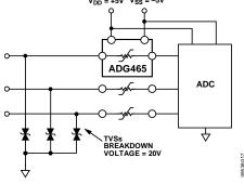
Figure 21. High Voltage Protection
