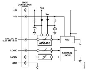
Figure 20. Overvoltage and Power Supply Sequencing Protection
