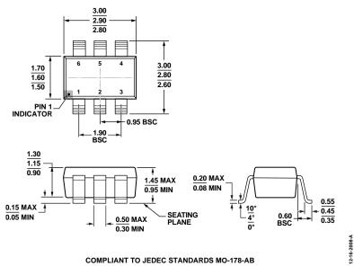
Figure 22. 6-Lead Small Outline Transistor Package [SOT-23] (RJ-6)
