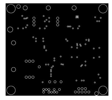
Figure 18. Layer 2 GND Plane
