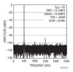
Figure 13. 16k Point FFT of the LTC2315-12 at  $f_{IN} = 500 \text{ kHz}$
