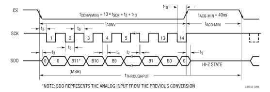
Figure 6: LTC2315-12 Serial Interface Timing Diagram (SCK High During taco)
