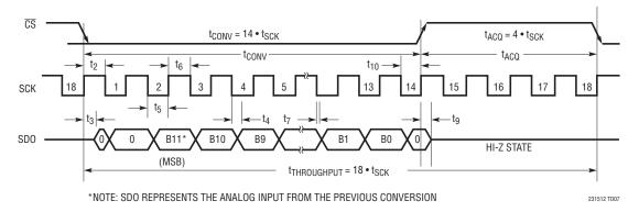
Figure 7: LTC2315-12 Serial Interface Timing Diagram (SCK Continuous)
