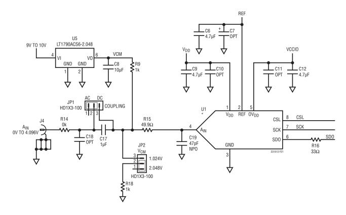
Figure 21. Partial DC1563 Demo Board Schematic
