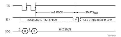
Figure 8: LTC2315-12 Entering/Exiting Nap Mode
