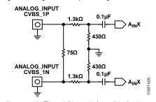
Figure 24. Differential Input Voltage Divider Network
