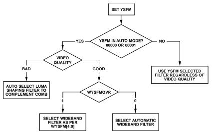
Figure 17. YSFM and WYSFM Control Flowchart
