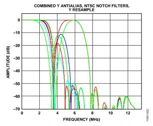
Figure 21. Combined Y Antialias Filter, NTSC Notch Filters
