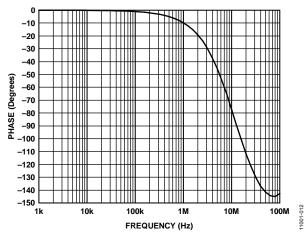
Figure 11. Antialiasing Filter Phase Response
