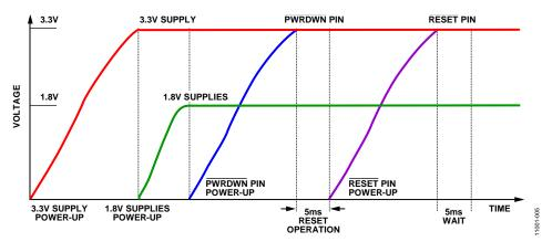
Figure 5. Recommended Power-Up Sequence
