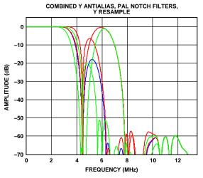
Figure 20. Combined Y Antialias, PAL Notch Filters
