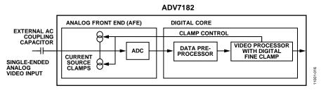
Figure 15. Single-Ended Clamping Overview
