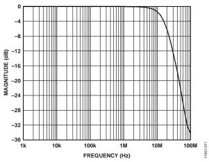
Figure 10. Antialiasing Filter Magnitude Response
