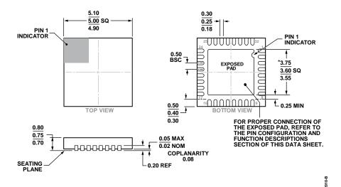
Figure 51. 32-Lead Lead Frame Chip Scale Package [LFCSP\_WQ] 5 mm × 5 mm Body, Very Very Thin Quad (CP-32-12) Dimensions shown in millimeters
