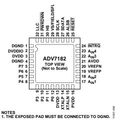
Figure 4. Pin Configuration
