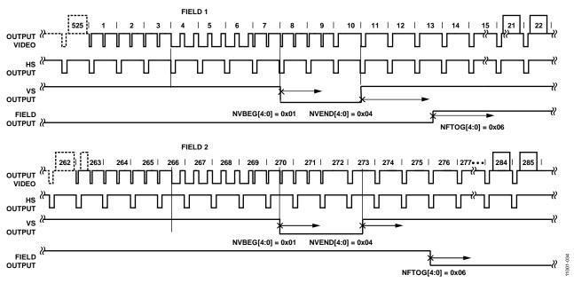
Figure 33. NTSC Typical VS/FIELD Positions
