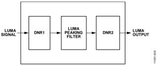
Figure 27. DNR and Peaking Block Diagram
