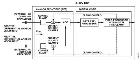
Figure 16. Differential Clamping Overview
