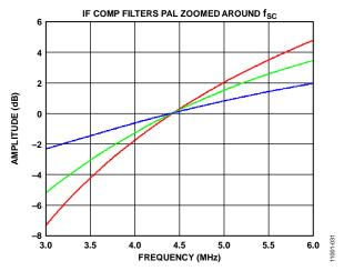
Figure 30. PAL IF Filter Compensation
