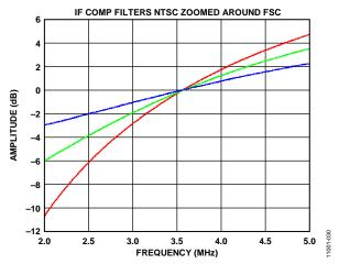
Figure 29. NTSC IF Filter Compensation
