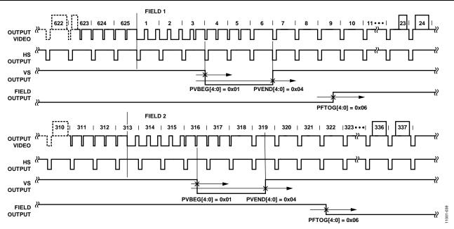
Figure 38. PAL Typical VS/FIELD Positions
