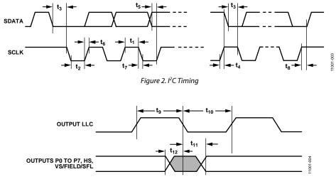
Figure 3. Pixel Port and Control Output Timing
