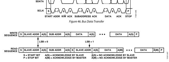
Figure 47. Read and Write Sequence
