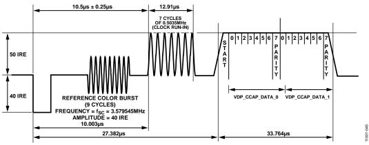
Figure 44. CCAP Waveform and Decoded Data Correlation
