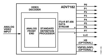
Figure 45. ITU-R BT.656 Output Stage of the ADV7182
