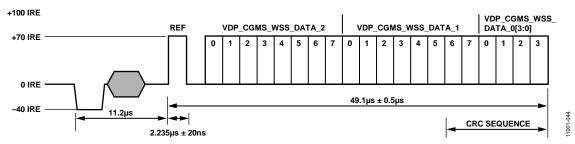
Figure 43. CGMS Waveform
