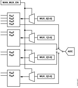
Figure 8. Manual Muxing
