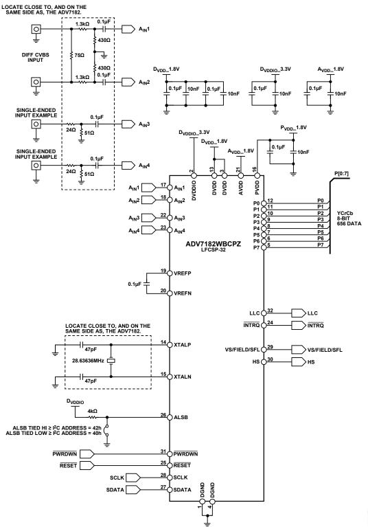
Figure 50. ADV7182 Typical Connection Diagram
