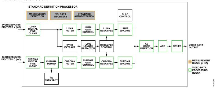
Figure 12. Block Diagram of Video Processor
