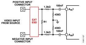
Figure 7. Input Differential Network
