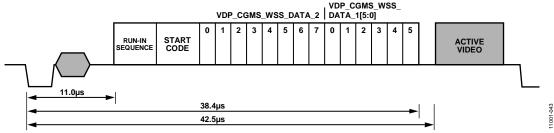
Figure 42. WSS Waveform
