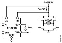
Figure 36. High-Side Current Sensing in Motor Control
