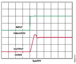
Figure 12. Rise Time (Differential Input = 200 mV)
