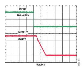
Figure 16. Differential Overload Recovery, Falling
