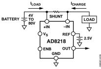
Figure 29. Operation with No Vs Connection
