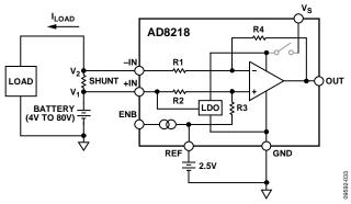
Figure 34. Bidirectional Operation Using a 2.5 V Reference Input
