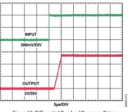
Figure 15. Differential Overload Recovery, Rising
