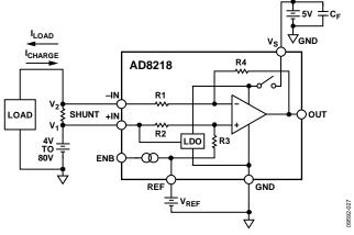
Figure 28. Simplified Schematic
