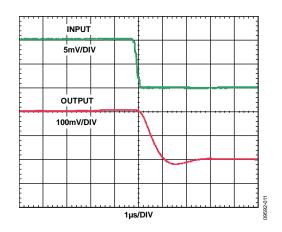
Figure 13. Fall Time (Differential Input = 10 mV)
