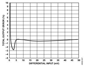
Figure 8. Total Output Error vs. Differential Input Voltage
