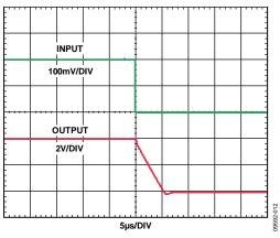
Figure 14. Fall Time (Differential Input = 200 mV)
