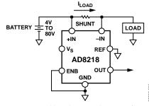
Figure 31. Enabling the Internal 80 mV Reference
