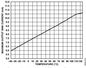
Figure 18. Maximum Output Sink Current vs. Temperature
