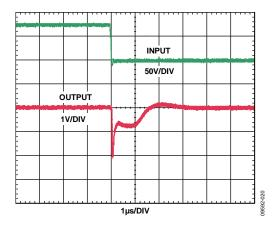
Figure 23. Common-Mode Step Response, Falling
