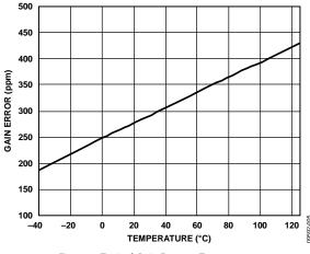
Figure 6. Typical Gain Error vs. Temperature
