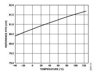
Figure 17. Internal Reference Voltage vs. Temperature ( $V_S = 5 V$ ,  $V_S = NC$ ,  $V_{CM} = 12 V$ , Pin 1 (+IN) and Pin 8 (–IN) Shorted, Pin 3 (ENB) Shorted to Pin 4 (GND))
