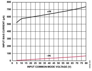
Figure 9. Input Bias Current vs. Input Common-Mode Voltage (Differential Input Voltage = 5 mV, V<sub>s</sub> = NC)
