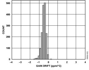
Figure 25. Gain Drift Distribution
