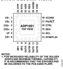
Figure 3. Pin Configuration
