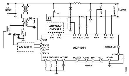
Figure 45. Active Clamp Forward Converter
