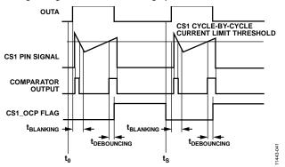
Figure 40. CS1 Cycle-by-Cycle Current-Limit Timing
