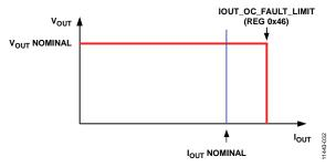
Figure 31. Constant Current Mode (Vout vs. Iout)
