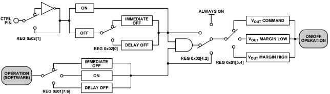
Figure 28. On/Off Control Diagram
