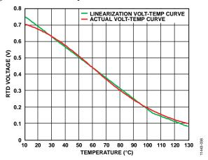
Figure 37. Temperature Linearization Scheme Curves
