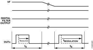
Figure 23. Closed-Loop Input Voltage Feedforward Changes Modulation
