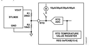
Figure 35. Temperature Sensing by an Analog Temperature Sensor
