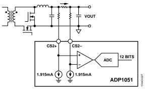
Figure 27. CS2 High-Side Resistive Current Sense
