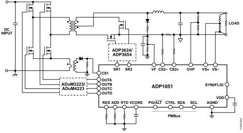
Figure 43. Full Bridge Converter
