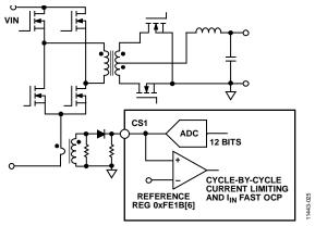
Figure 25. Current Sense 1 (CS1) Operation
