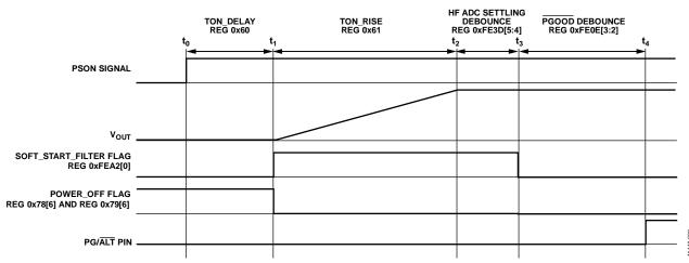
Figure 29. Soft Start Timing Diagram
