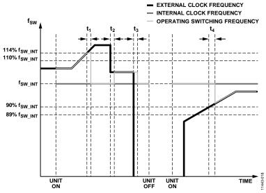
Figure 17. Synchronization Operation
