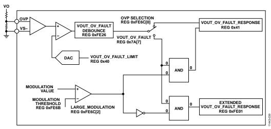
Figure 38. Vout Overvoltage Protection Circuit Implementation
