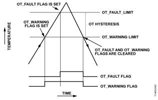
Figure 39. OT Protection and OT Warning Operation
