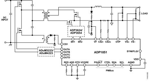
Figure 44. Half Bridge Converter
