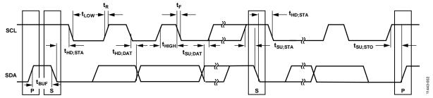
Figure 2. Serial Bus Timing Diagram
