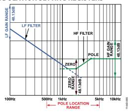
Figure 66. Digital Compensator Programmability
