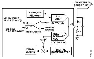
Figure 22. Closed-Loop Input Voltage Feedforward Configuration
