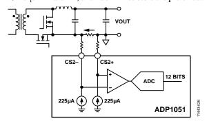
Figure 26. CS2 Low-Side Resistive Current Sense
