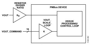
$\textit{Figure 63. Conceptual View of the VOUT\_SCALE\_LOOP\ Command}$
