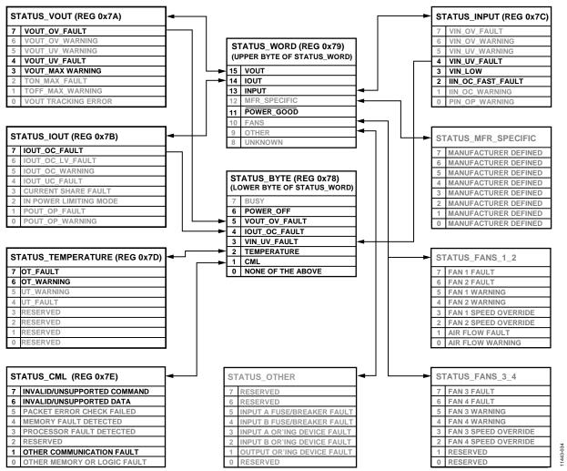
Figure 33. Summary of the Fault Status Registers (Only the commands in black are supported by the ADP1051; the commands in gray are not supported.)
