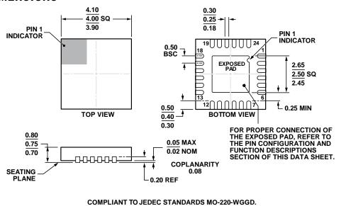
Figure 69. 24-Lead Lead Frame Chip Scale Package [LFCSP] 4 mm × 4 mm Body and 0.75 mm Package Height (CP-24-15) Dimensions shown in millimeters
