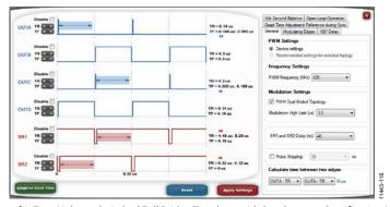
Figure 13. PWM Settings for Zero-Voltage-Switched Full Bridge Topology with Synchronous Rectification Using the ADP1051 GUI Rev. B | Page 15 of 108
