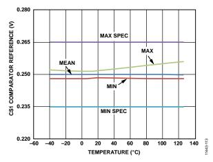
Figure 10. CS1 OCP Comparator Reference vs. Temperature (0.25 V Reference)
