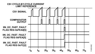
Figure 41. I<sub>IN</sub> Overcurrent Fast Fault Triggering
