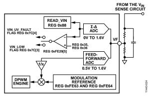
Figure 24. Open-Loop Feedforward Operation
