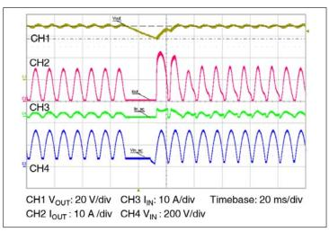
Figure 13 – Line drop out, 50 Hz, 0° phase,  $V_{IN}$  = 240 V,  $P_{LOAD}$  = 330 W,  $C_{OUT}$  = 12,000  $\mu F$ .
