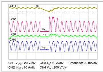
**Figure 14** – Line drop out, 50 Hz, 90° phase,  $V_{IN}$  = 240 V,  $P_{LOAD}$  = 330 W,  $C_{OUT}$  = 12,000  $\mu$ F.
