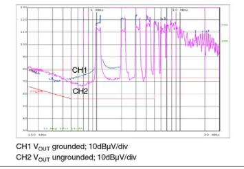
Figure 15 – Typical EMI spectrum, full load, unfiltered,  $V_{IN} = 120 \text{ V}, C_{OUT} = 12,000 \text{ }\mu\text{F}.$
