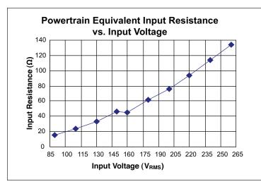
**Figure 22 –** Dynamic input resistance vs.  $V_{IN}$ ,  $I_{OUT} = 6.9$  A.
