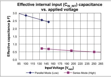
**Figure 23 –** Effective input capacitance vs.  $V_{IN}$ .
