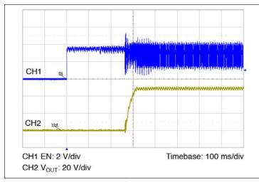
**Figure 12 –** Typical startup waveform, EN pin release,  $V_{IN}$  = 240 V,  $R_{LOAD}$  = 7.1  $\Omega$ ,  $C_{OUT}$  = 12,000  $\mu$ F.
