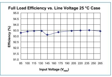
Figure 2 — Full load efficiency vs. line voltage
