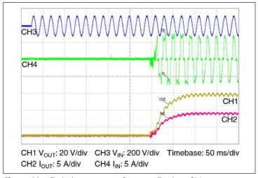
**Figure 11 –** Typical startup waveform, application of  $V_{IN}$ ,  $R_{LOAD} = 7.1 \ \Omega$ ,  $C_{OUT} = 12,000 \ \mu F$ .
