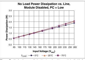
**Figure 7 –** No load power dissipation trend vs.  $V_{IN}$ , module disabled.
