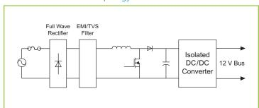
Figure 27 - Traditional PFC AC to DC supply
