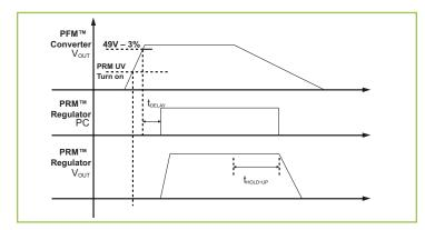
Figure 31 – PRM Enable Hold off Waveforms
