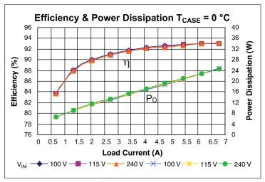
**Figure 19** –  $V_{IN}$  to  $V_{OUT}$  efficiency and power dissipation vs.  $V_{IN}$  and  $I_{OUT}$ ,  $T_{CASE} = 0$ °C.
