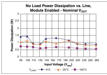
**Figure 6** – Typical no load power dissipation vs.  $V_{IN}$ , module enabled.
