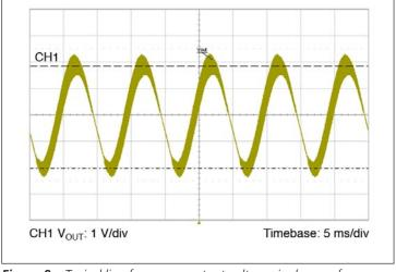
**Figure 9 –** Typical line frequency output voltage ripple waveform,  $T_{CASE}=30$  °C,  $V_{IN}=230$  V,  $I_{OUT}=6.9$  A,  $C_{OUT}=6.000$   $\mu F$ .
