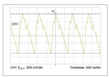
**Figure 8** – Typical switching frequency output voltage ripple waveform,  $T_{CASE} = 30$  °C,  $V_{IN} = 230$  V,  $I_{OUT} = 6.9$  A, no external ceramic capacitance.
