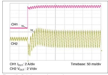
**Figure 10** – Typical output voltage transient response,  $T_{CASE} = 30$  °C,  $V_{IN} = 230$  V,  $I_{OUT} = 6.9$  A,  $C_{OUT} = 6,000$   $\mu$ F.
