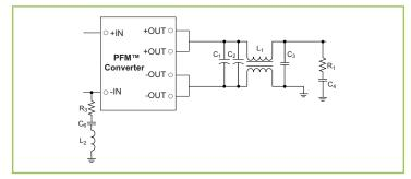
**Figure 29 –** Typical filter schematic (positive output)
