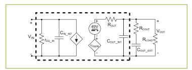
Figure 28 - PF175B480C033FP-00 AC small signal model
