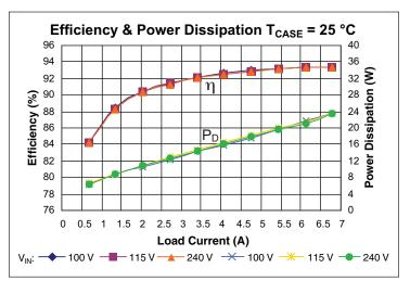
**Figure 20** – Line to  $V_{OUT}$  efficiency and power dissipation vs.  $V_{IN}$  and  $I_{OUT}$ ,  $T_{CASF} = 25$ °C.
