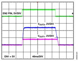
Figure 24. Coincident Voltage Tracking Response
