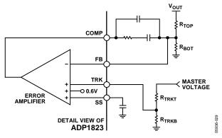
Figure 30. Voltage Tracking
