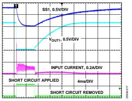
Figure 17. Output Short-Circuit Response
