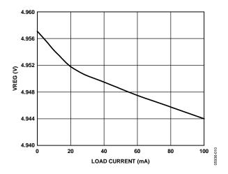
Figure 10. VREG vs. Load Current,  $V_{IN} = 12 V$
