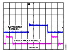
Figure 18. Out-of-Phase Switching, Internal Oscillator
