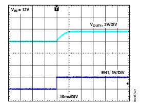
Figure 21. Enable Pin Response,  $V_{IN} = 12 V$
