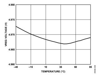
Figure 8. VREG Voltage vs. Temperature
