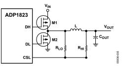
Figure 25. Short-Circuit Current Foldback Scheme
