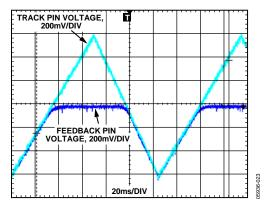
Figure 23. Output Voltage Tracking Response
