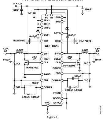
component size and cost. For noise sensitive applications, it can also be synchronized to an external clock to achieve switching frequencies between 300 kHz and 1 MHz. The ADP1823 includes soft start protection to prevent inrush current from the input supply during startup, reverse current protection during soft start for precharged outputs, as well as a unique adjustable lossless current-limit scheme using external MOSFET sensing.
