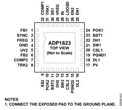
Figure 3. Pin Configuration
