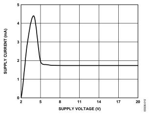
Figure 15. Supply Current vs. Supply Voltage
