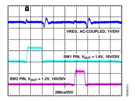
Figure 12. VREG Output During Normal Operation
