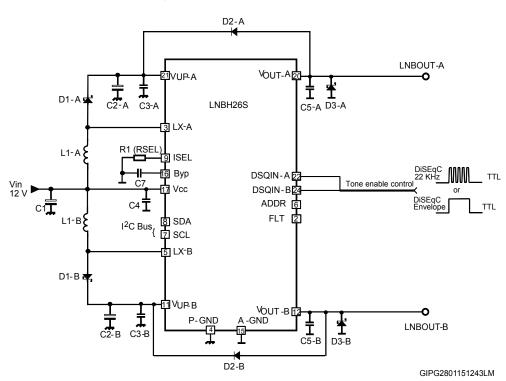
Figure 6. DiSEqC 1.x application circuit
