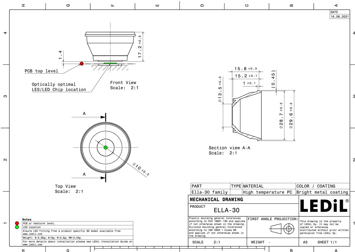
See also our general installation guide: [www.ledil.com/installation\\_guide](http://www.ledil.com/installation_guide)
