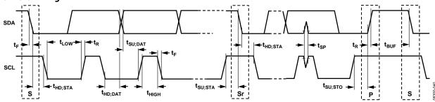
Figure 65. I<sup>2</sup>C Serial Port Timing
