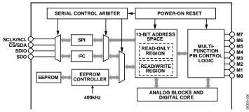
Figure 51. Serial Port Functional Diagram
