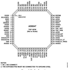
Figure 2. Pin Configuration
