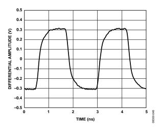
Figure 23. Output Waveform, LVDS (400 MHz)
