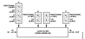
Figure 40. Third-Order Digital IIR Loop Filter
