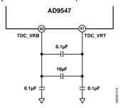
Figure 38. TDC Pin Connections
