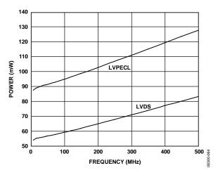
Figure 15. Power Consumption vs. Frequency, LVPECL and LVDS (Single Channel)
