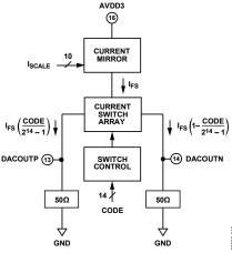
Figure 43. DAC Output Pins
