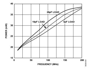
Figure 18. Power Consumption vs. Frequency, 1.8 V CMOS
