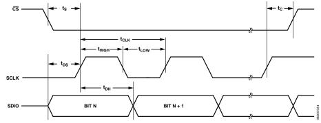
Figure 59. Serial Control Port Timing—Write
