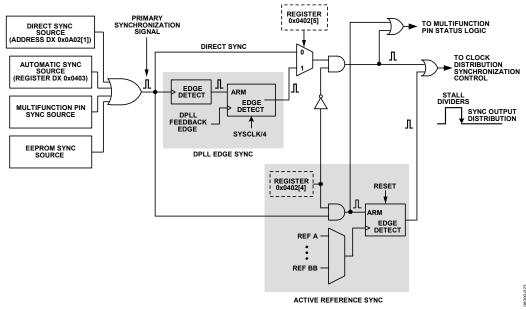
Figure 48. Output Synchronization Block Diagram
