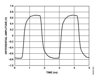
Figure 20. Output Waveform, LVPECL (400 MHz)
