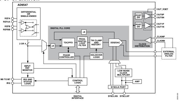
Figure 33. Detailed Block Diagram
