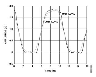
Figure 25. Output Waveform, 1.8 V CMOS (100 MHz)
