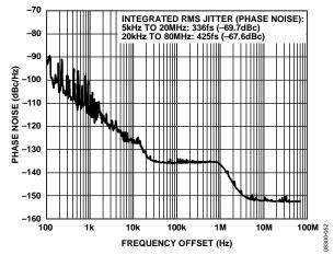
Figure 11. Absolute Phase Noise (Output Driver = LVPECL),  $f_{\rm REF} = 8$  kHz,  $f_0 = 155.52$  MHz, LBW = 100 Hz,  $f_{\rm SYSCLK} = 50$  MHz (Crystal), PLL On
