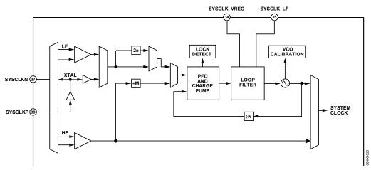
Figure 45. System Clock Block Diagram
