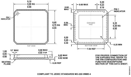
Figure 69. 64-Lead Lead Frame Chip Scale Package [LFCSP\_VQ] 9 mm × 9 mm Body, Very Thin Quad (CP-64-4) Dimensions shown in millimeters
