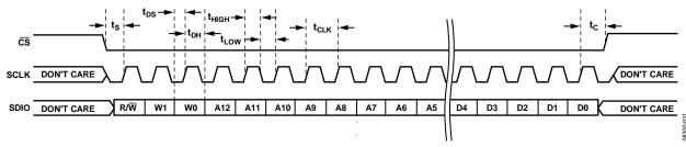
Figure 56. Serial Control Port Write—MSB First, 16-Bit Instruction, Timing Measurements
