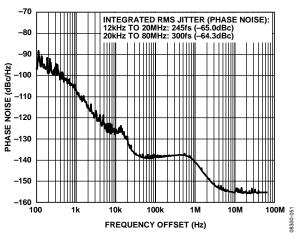
Figure 8. Absolute Phase Noise (Output Driver = LVPECL),  $f_{REF} = 19.44$  MHz,  $f_0 = 155.52$  MHz, LBW = 1 kHz,  $f_{SYSCLK} = 50$  MHz (Crystal), PLL On with  $2 \times$  Frequency Multiplier,  $I_{CP} = 375$   $\mu$ A, LF = External (350 kHz)
