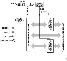
Figure 66. Buffered and Active Registers
