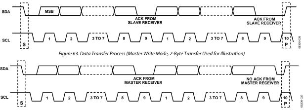
Figure 64. Data Transfer Process (Master Read Mode, 2-Byte Transfer Used for Illustration)
