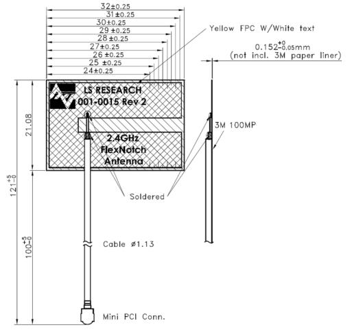
Figure 1: FlexNotch mechanical drawing
