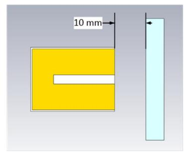
Figure 18: Open side metal clearance
