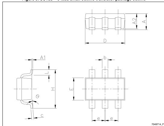
Figure 9. SOT23 - 6-lead small outline transistor package outline
