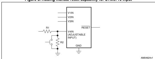
Figure 8. Adding manual reset capability for STM6710 input
