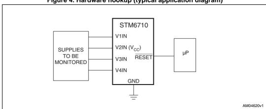
Figure 4. Hardware hookup (typical application diagram)
