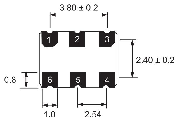
**Package is Seam Sealed Ceramic-Metal.**
