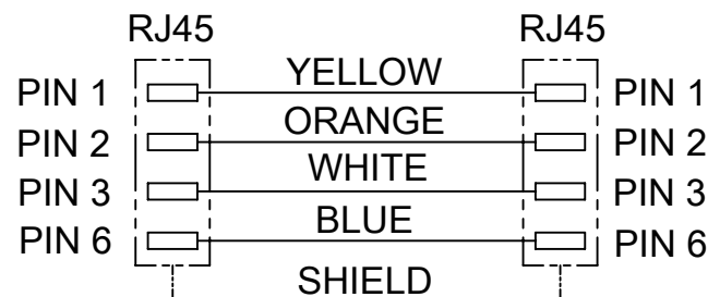
WIRING DIAGRAM FOR CABLE TYPE 11, 12
