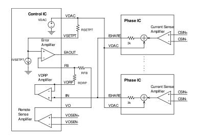
Figure 9 - Adaptive voltage positioning
