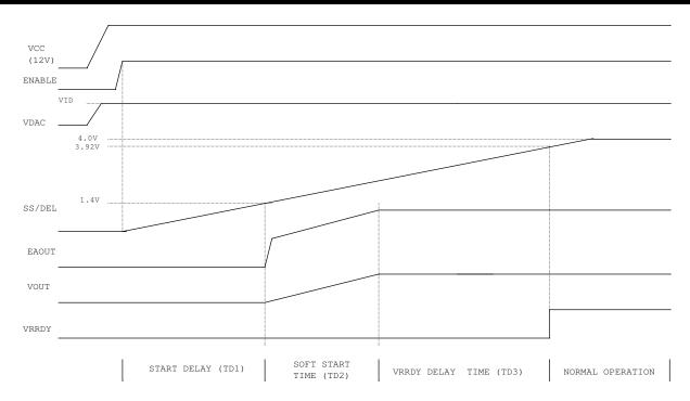
Figure 12 - Start-up sequence of converter without boot voltage
