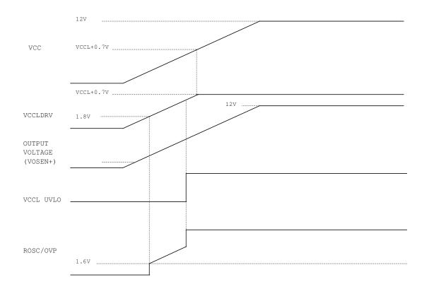
Figure 16 - Over-voltage protection during power-up
