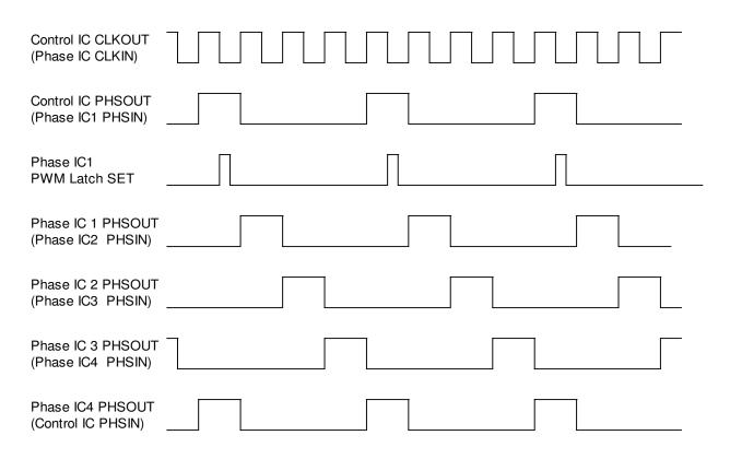
Figure 5 - Four Phase Oscillator Waveforms
