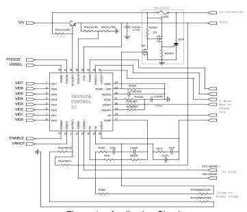
Figure 1 – Application Circuit
