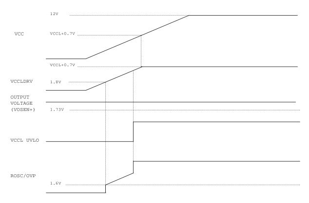
Figure 17 - Over-voltage protection with pre-charging converter output Vo > 1.73V
