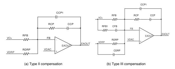
Figure 22 - Voltage loop compensation network
