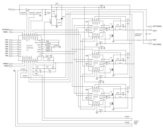
Figure 20 - IR3500A / IR3505 Three Phase AMD Opteron Converter
