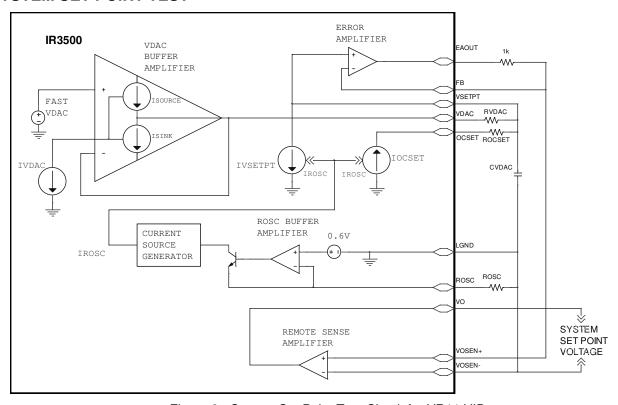
Figure 2 - System Set Point Test Circuit for VR11 VID
