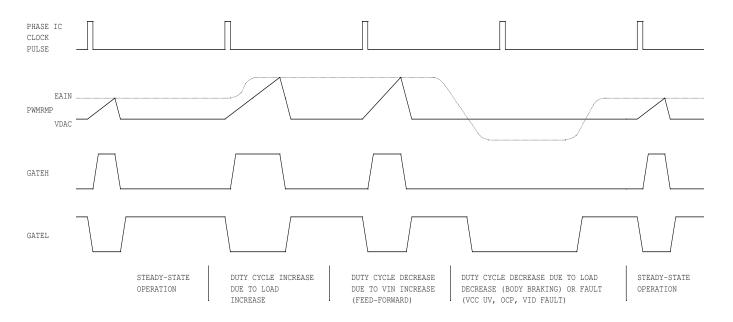
Figure 6 - PWM Operating Waveforms
