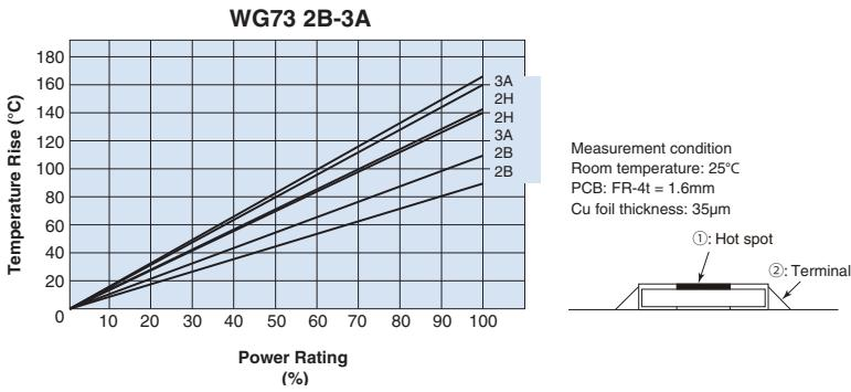
Regarding the temperature rise, the value of the temperature varies per conditions and board for use since the temperature is measured under our measuring conditions.
