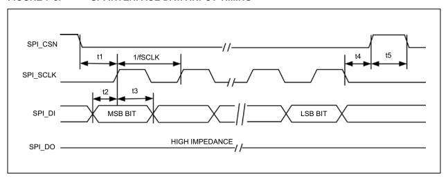
FIGURE 7-9: SPI INTERFACE DATA OUTPUT TIMING
