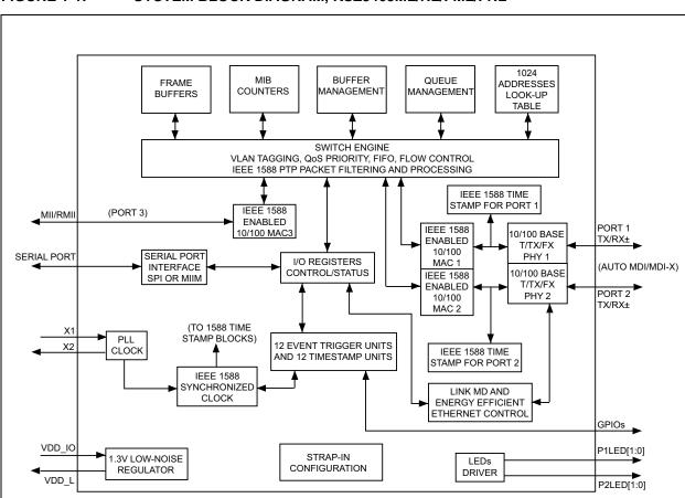
FIGURE 1-1: SYSTEM BLOCK DIAGRAM, KSZ8463ML/RL/FML/FRL
