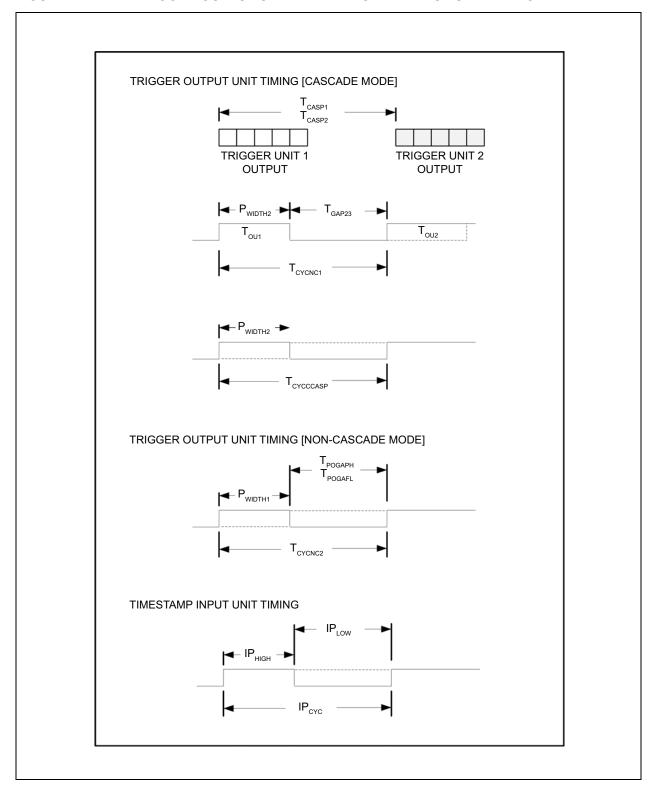
TABLE 7-9: TRIGGER OUTPUT UNIT AND TIME STAMP INPUT UNIT TIMING PARAMETERS
