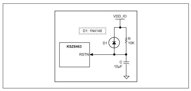
The following reset circuit is recommended for applications where reset is driven by another device (e.g., CPU or FPGA). At POR, R, C and D1 provide the necessary ramp rise time to reset the KSZ8463 device. The RST\_OUT\_N from CPU/FPGA provides the warm reset after power-up.
