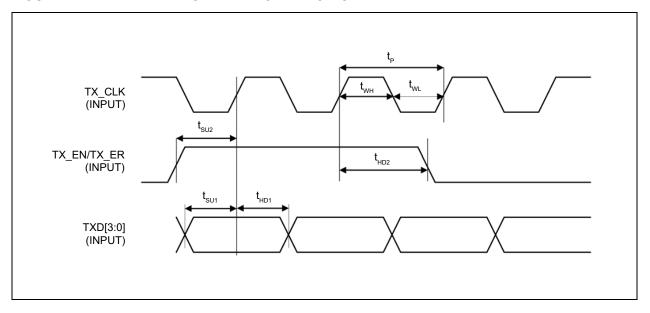
TABLE 7-1: MII TRANSMIT TIMING IN MAC MODE PARAMETERS
