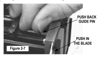
**Note:** The prismatic blades must be installed so they overlap when closed.
