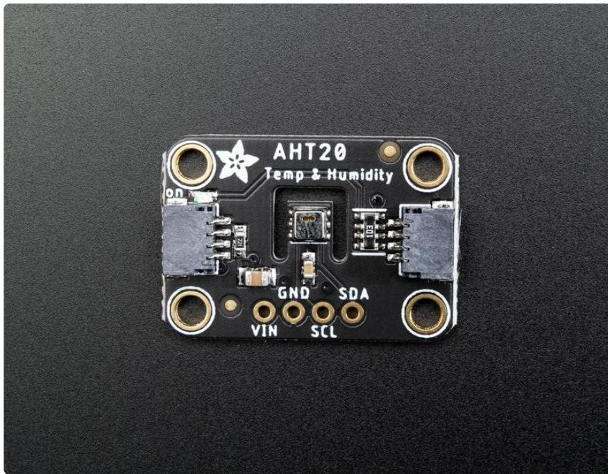
The AHT20 is a nice but inexpensive temperature and humidity sensor [from the same folks that brought us the DHT22](#) (<https://adafru.it/sb4>). You can take sensor readings as often as you like, and it uses standard I2C so its super easy to use with any Arduino or Linux/Raspberry Pi board.
