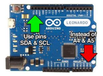
Because UNTZtrument is based around the Arduino Leonardo, it requires slightly different wiring: Use the SDA and SCL pins instead of A4 and A5 as shown in the guide.
