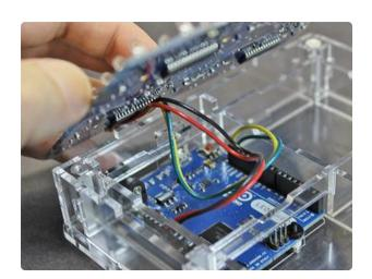
Now get the Trellis board ready. Remove the rubber buttons for the time being and turn the board face-down.
