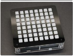
Install the clear top "waffle" piece. Since you'll still be holding the Trellis down, start from one edge, aligning the notches with the tabs on the side pieces, and swing this down into place as you remove your other hand.
