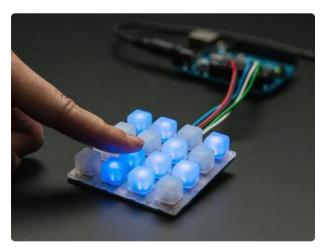
UNTZtrument is based on Adafruit's Trellis, a 4x4 backlit keypad kit.
