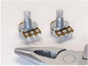
If adding more than one potentiometer, the legs must be bent back to fit inside the case. If two potentiometers are installed in the same quadrant, they install back-to-back.
