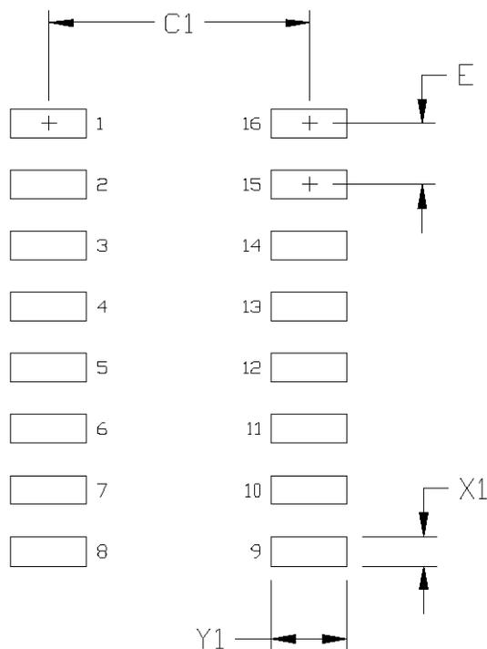
**Figure 12.1. 16-Pin Narrow Body SOIC PCB Land Pattern**
