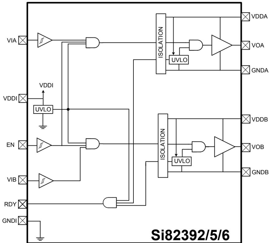
Figure 5.2. Si82392/5/6 Dual Isolated Drivers with RDY Pin
