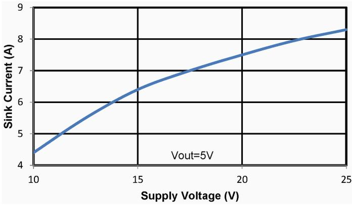
Figure 2.11. Output Sink Current vs. Supply Voltage
