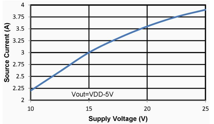
Figure 2.12. Output Source Current vs. Supply Voltage
