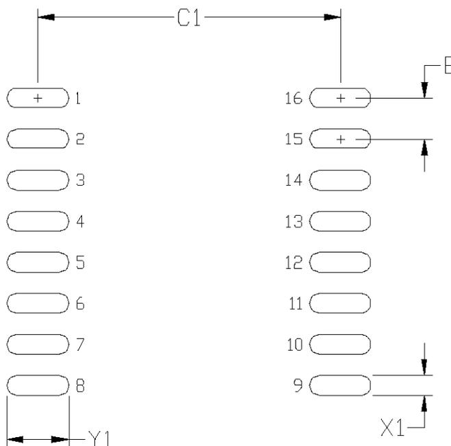
**Figure 10.1. 16-Pin Wide Body SOIC PCB Land Pattern**
