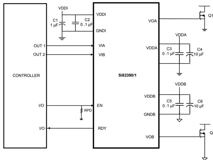
Figure 3.4. Si82390/1 with Enhanced UVLO Feature Application Diagram
