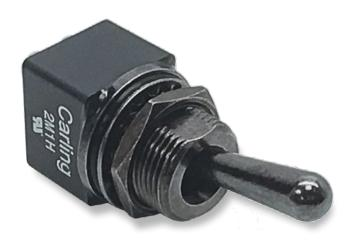
The 2M family of miniature toggle switches is composed of three switch series; the 2M1-Series miniature toggle switch, the 2MS-Series sealed miniature toggle switch, and the 2M1H-Series premium sealed miniature toggle switch. These series all feature PC mounting and offer a variety of ratings, circuits, contact materials, terminal platings, toggle styles and lengths, and optional color caps.
