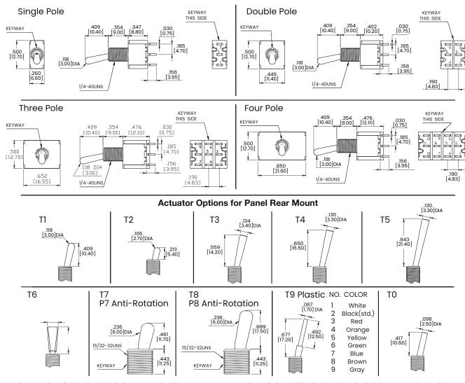
\* T6 actuator is available with B1, B2, B5, B6, BA, BB & BE bushing. Actuator length shown for T1-T5,T9 and T10 is with B1 bushing. T7, P7, P8 does not require a bushing code.
