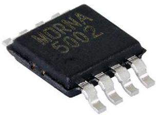
MORN series resistor networks feature four isolated resistors with standard 0.65 mm (25.6 mil) pitch lead spacing. The networks feature close TCR tracking and tight ratio tolerance and are ideally suited for unity gain operational amplifier circuitry. The standard resistance offerings listed are available for immediate delivery.
