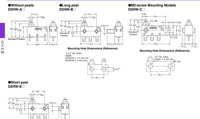
Note. The reference positions used for Free Position (FP), Operating Position (OP), and Total Travel Position (TTP) values are as shown above for each type of mounting.
