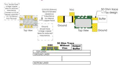
Attention: To achieve optimal frequency stability, and in some cases to meet the specification stated on this data sheet, it is required that the circuit connected to this TCXO output must have the equivalent input capacitance that is specified by the nominal load capacitance. Deviations from the nominal load capacitance will have a graduated effect on the stability of approximately 20 ppb per pF load difference.
