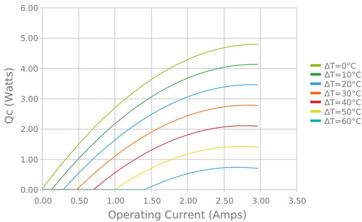
Heat Pumped at Cold Side
