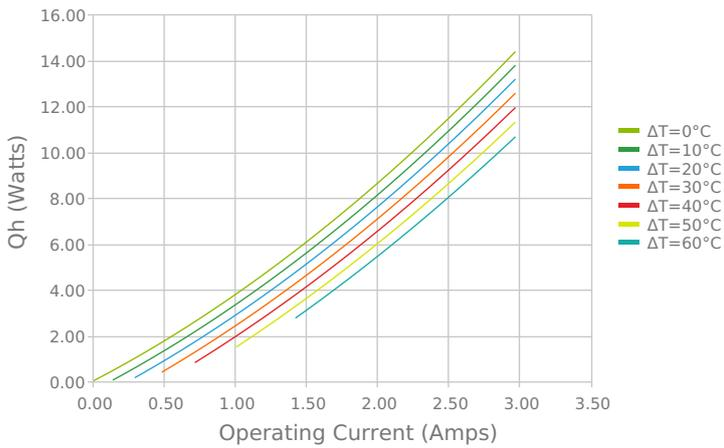
Total Heat Dissipated at Hot Side (Qh=Qc+Pin)
