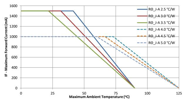
Figure 11: Maximum forward current vs. ambient temperature
