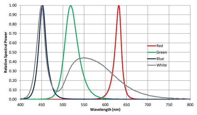
Figure 5: Typical relative spectral power vs. wavelength @  $T_c = 25^{\circ}C$ .
