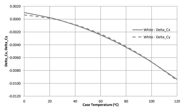
Figure 10b: Typical chromaticity coordinate shift vs. case temperature
