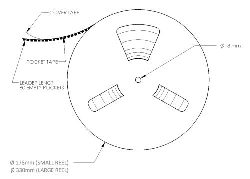
Figure 13: Emitter reel specifications (mm).
