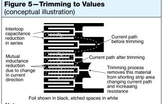
**Note**To acquire a precision resistance value, the Bulk Metal® Foil chip is trimmed by selectively removing built-in "shorting bars." To increase the resistance in known increments, marked areas are cut, producing progressively smaller increases in
