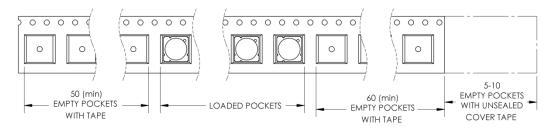
Figure 12: Emitter carrier tape specifications (mm).
