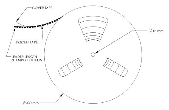
Figure 13: Emitter Reel specifications (mm).
