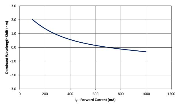
Figure 9: Typical dominant wavelength shift vs. forward current @  $T_c = 25^{\circ}C$ .
