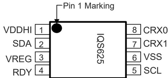
**Figure 1-1 Pin out of IQS625 TSSOP (3X6.4)-8 package.**
