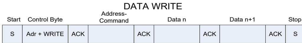
**Figure 5-4 I<sup>2</sup>C Write**
