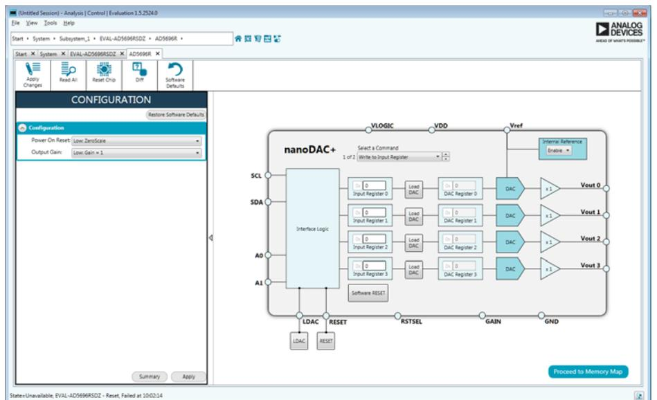
Figure 3. Chip Block Diagram of the [AD5696R](#)
