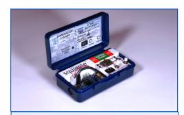
**Developer's kits** demonstrate system performance of an integrated SQUIGGLE motor, NSD-2101 driver and NSE-5310 position sensor.
