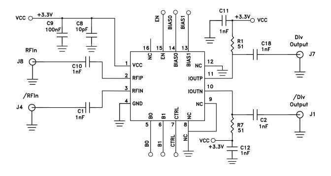
Input Voltage Range 3.15V min, 3.3V nom, 3.45 V max Current 80mA to 125mA
