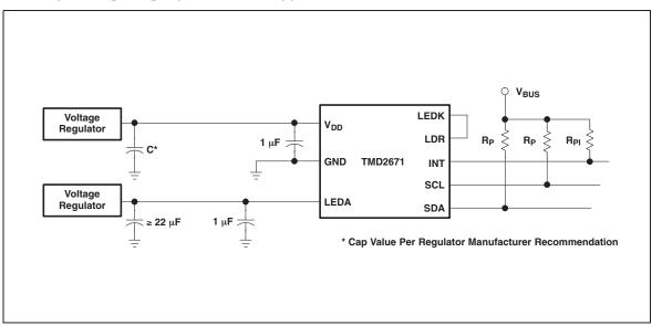
If it is not possible to provide two separate power supplies, the device can be operated from a single supply. A  $22\Omega$  resistor in series with the  $V_{DD}$  supply line and a  $1\mu F$  low ESR capacitor effectively filter any power supply noise. The previous capacitor placement considerations apply.
