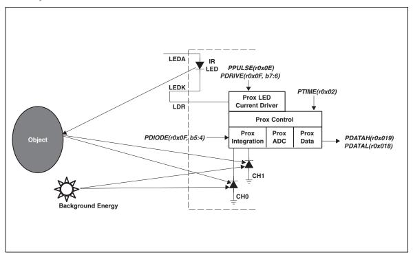
The LED current driver provides a regulated current sink on the LDR terminal that eliminates the need for an external current limiting resistor. The PDRIVE register setting sets the sink current to 100%, 50%, 25%, or 12.5% of the factory trimmed full scale current.
