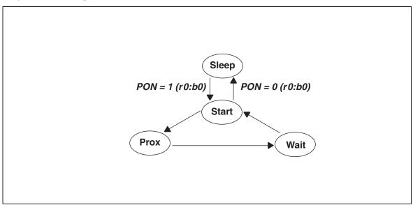
**Note:** In this document, the nomenclature uses the bit field name in italics followed by the register number and bit number to allow the user to easily identify the register and bit that controls the function. For example, the power on (PON) is in register 0, bit 0. This is represented as *PON* (*r0:b0*).
