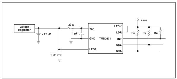
$V_{BUS}$  in the above figures refers to the  $I^2C$  bus voltage which is either  $V_{DD}$  or 1.8V. Be sure to apply the specified  $I^2C$  bus voltage shown in the Ordering Information table for the specific device being used.
