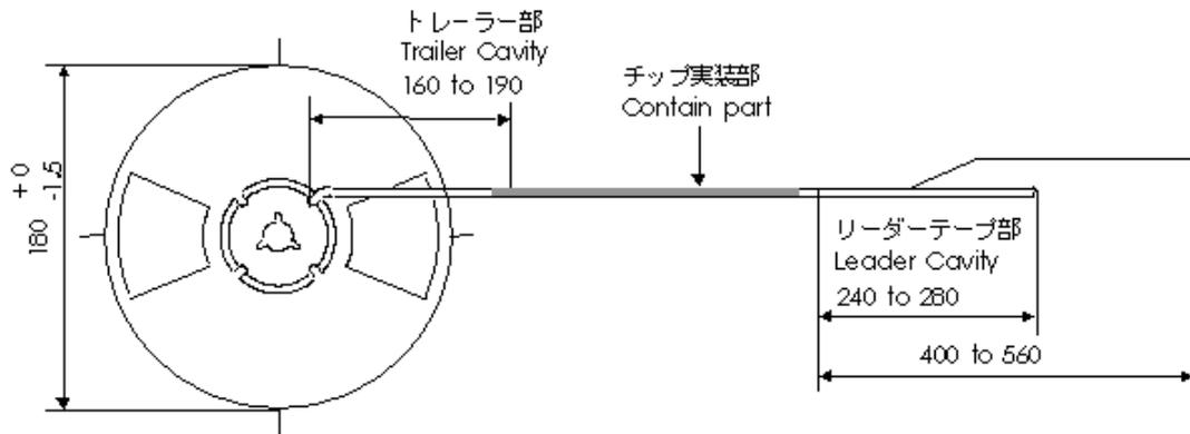
The tape for transducer shall be wound clockwise. The feeding holes shall be to the right side as the tape is pulled toward the user.
