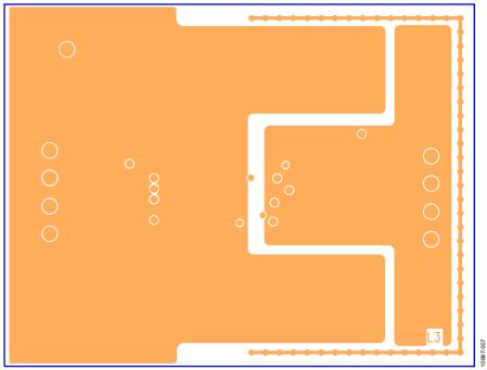
Figure 6. EVAL-ADM3252EEBZ Internal Layer 3
