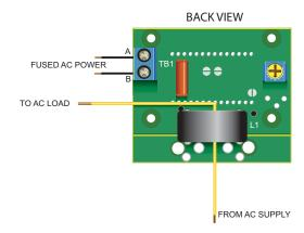
Figure 2. Connections for pc-board mounted CT's
