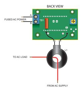
Figure 3. Connection for flying lead CT's
