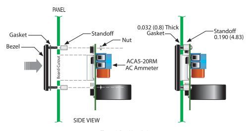
Figure 4. Panel Installation
