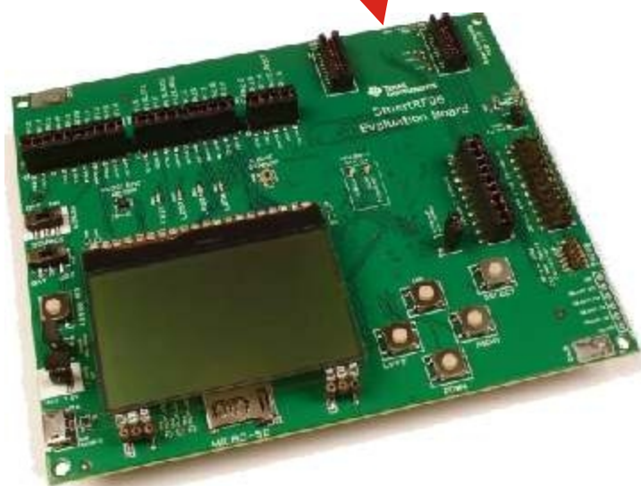
SMART RF06 Evaluation board (TI)
